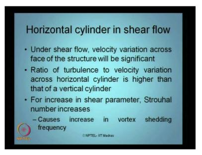
So, they will also be subjected to flow induced vibration in addition to the inline and transverse vibrations happening because of the wave interaction. If I talk about, the horizontal flow cylinders in a shear flow because we saw in the vertical cylinder in the shear flow.
