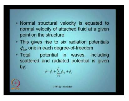
So, Normal structure velocity is now, calculate in all degrees of freedom as you see this expression here, which is included the scattered potential and radiated potential both are and s as well. So, phi rk what is see here, is a force oscillation of unit amplitude which is worked out for every degree freedom where k is the each degree of freedom separately.
