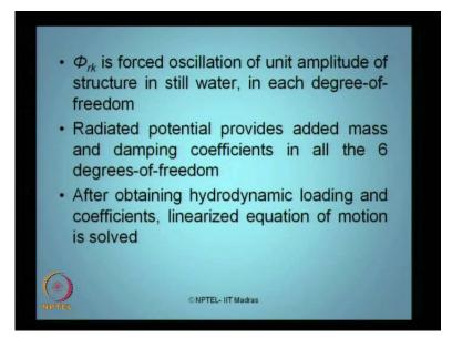
So, radiated potential provides added mass and damping coefficient for my analysis in all the 6 degrees-of-freedom separately. So, after obtained hydrodynamic loading obtained in the member, linear equation of motion which is been solved using different techniques either in time domain or in frequency domain. That is how, my dynamic analysis of incorporating the FSI in structural problem where this cylinder is fixed or it is a large in diameter or this floating.
