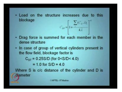
So, load on structure increases because of this reduced velocity due to this blockage, and we compute this blockage factor as CBF as given in this expression where the drag force on each member is summed up separately and then arrived at, for the influence of blockage factor on the structures.
