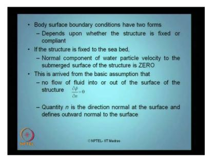
So, now the body surface Boundary condition has two forms which depends slowly, on the structure where the fixed or compliant we will see both the case of now. When the structure is fixed to the sea bed the normal component as you just saw, of the water particle velocity to the submerged surface of the structure remain 0. So, this arrived in the basic assumption that the derivative of the potential with respect to the directionality normal remain 0.
