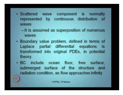
The scattered wave component is generally represented by continuous distribution of waves, because it keeps on scattering all directions as far as instance wave is concerned when it encounter cylinder, but it is assumed to be superposition of numerous waves using a specific theory.
