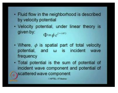
So, the fluid flowing the neighborhood is described a Velocity potential as given in this expression under linear theory, where in this case phi is the special part of the Total velocity potential the special variation created in the velocity potential where is omega is the frequency of the instance wave which you already know, what is fitting or what is encountering the vessel or the cylinder.
