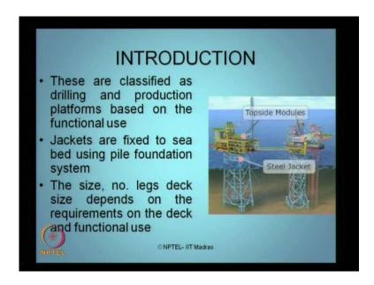
It is very important that in case of offshore structures, this combination, the integral and unique value of combining them together, whereas, possibly I think, offshore structures are one amongst the unique combination, where common function both are combined together to arrive at the structural system. No other system has this kind of uniqueness.
