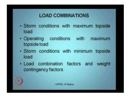
So, we also look at the different load combinations. The storm condition with maximum topside load, that is, one combination and the operation condition has maximum topside load. Of course, the storm conditions with minimum topside load and the load combination factors with the weighted contingency factors are available on the design.
