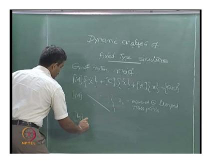
In this lecture, in module 2, we will talk about the dynamic analysis of fixed type structures. So, as we all understand, the classical equation of motion for any multi degree freedom system model is given by. It is a classical equation of motion, where mass matrix generally is diagonal of the limits are not present, provided the degrees of freedom are measured at the lumped mass points and k can be derived from the first principle.
