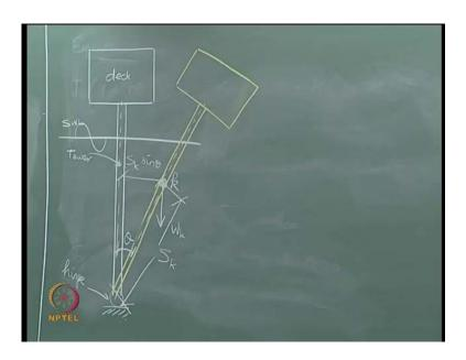
So, I pick up any element here, which is K, I call this length of the element from the hinge as S K on the element has W K as weight. Now, of course, we know this value will be S K sin theta.
