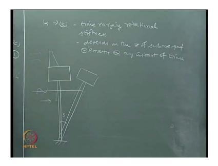
Whereas K nu T is again a time varying rotational stiffness, it is a times varying rotational stiffness, this depends on the number of submerge elements at any instant of time. Whereas K is the rotational stiffness at undisplaced position, I think you will understand at now, when I apply lateral force to this tower, when I have a tower this form is single tower hinge at the bottom subjected to wave action.
