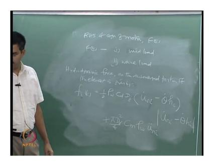
The second force of course, we have is the wave load. We will try to slightly expand this, because I need this to expand it for understand the scheme of solutions procedure for this problem. So, we already know the hydrodynamics force on the submerged proportion of the element is given by let us say f i of t, I am using, I here, I will explain what I is half rho C d D of the j th element is given by j th element.
