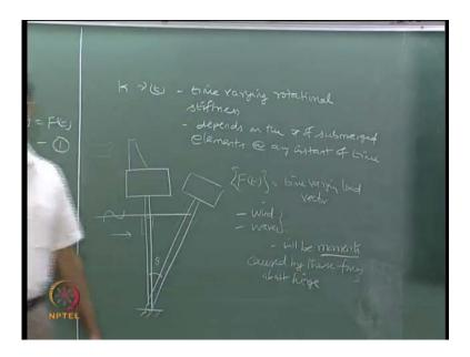
Now, of course, F of T, it is the time varying vector, time varying load vector, which in this case arise from wind and waves both are consider in this analysis. And in this essentially, F of T will be the moments caused by this forces about hinge, not the load actually, it is a moment. That is a moment caused various forces above the sea. So, let me re write this equation again here.
