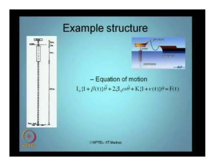
So, what we do is we pick up a tower, we see in the left hand side here and you can see, there are discretized points, which has been dividing these towers into various components. So, the height of the tower the physical dimension about 275 meters and then the buoyancy tank is about 70 meter deep, which is located close to M S L or the still water level.
