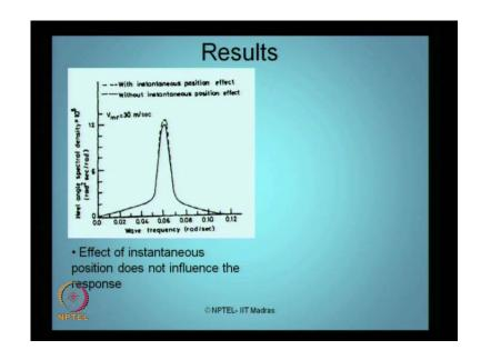
Again, the expectation is seen only in the narrow band over let us say 0.045 the 0.075 wherein, the max velocity of the wind energy is being concentrated and the variation is not, the reasoning is gain same the non-linear effect are not significant because the system is too flexible.
