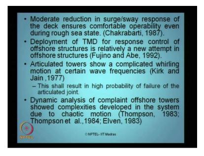
So, based on these people suggested in 1994 an idea that why cannot we use tuned mass dampers, tuned mass dampers TMD for response control. So, this is the first time people thought yes! Let me control the response using the different external mechanism where, I can tune my secondary mass to the primary mass using principles of dynamics to control the response. So, what we call as tuned mass dampers.
