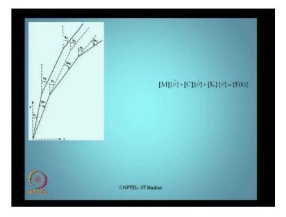
Let us derive the equation of motion for this very quickly and see how equation of motion looks like for this tower. Any question here? So, I am drawing this figure back again anyway, I am drawing it here, may not have to see it, here I am going to draw this figure again.
