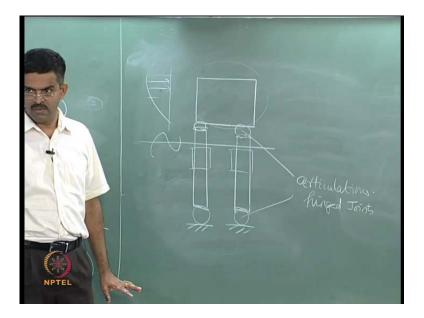
So, I have a tower now, which is comprising a deck which is again having the columns now, I am drawing 2 in elevation. So, I am introducing a new element here of course, this element already is present so, both are articulation nothing but, hinged joints. Now, one can wonder why this fundamental deviation from a single tower. The fundamental deviation was made from a single tower because the single tower demonstrated a rigid body motion.
