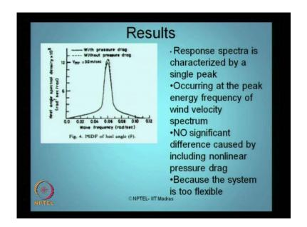
So, that analysis has been imposed on this particular tower and the results are the following. So, there is figure which shows the power spectral density function of the heel angle theta which is plotted for different frequency band varying from 0 to 0.12.
