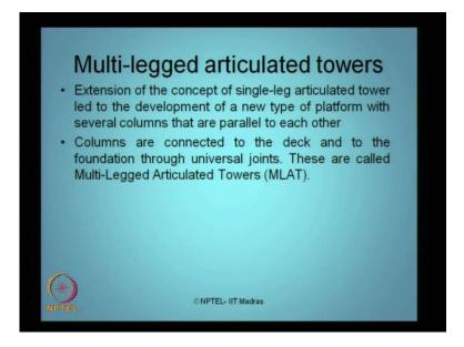
So, let us quickly see what are multi legged articulated towers which is abbreviated as MLAT is multi legged articulated towers. It is nothing but, the extension of the concept of single tower to the development of a new type of platform where there are several
