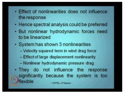
So therefore, the effect of nonlinearities does not influence the respond in this specific example. So, spectral analysis can be preferred for this case. So, non-linear
