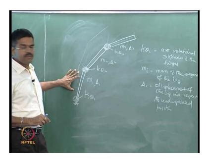
Let us say there are 3 hinges hinge: 1 hinge, 2 and hinge 3. I call this stiffness of this rotational stiffness of this spring as k theta, the rotational stiffness of this spring as k theta 2 and this as k theta 3 respectively. So, k theta i are the rotational stiffness of the hinges. Of course, m 1, m 2, m 3 are the respective mass. Delta 1, delta 2 and delta 3 are displacement of the length respect to vertical, undisplaced position. Un-displaced vertical, the bottom leg is vertical.
