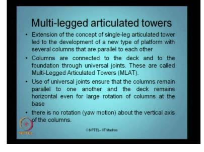
So, of course, use of universal joints enables the column to remain parallel to each other and the deck remains almost horizontal not exactly horizontal even for large rotation column at the base. This was not happening in the earlier case. We just now saw the rigid body motion is there between the tower and the deck. So, now this isolates the tower from the deck.
