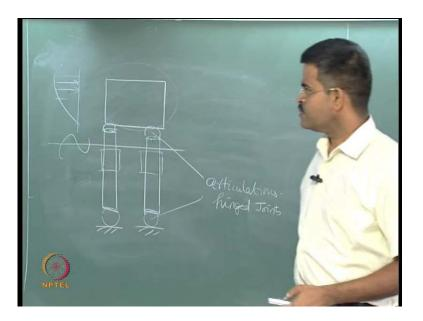
So, now they said let use have multi-legged towers, multi legged towers are actually legs parallel to each other and connected to the deck using a hinged joint.
