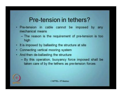
So, how pretension is imposed on the tether as you understand; how it is imposed on a guyed tower? There is a fare lead point; there is a fare lead point through which the cable passes and goes to the hull there are lock lot of rock, rocker mechanic systems kept on the hull on the top, which will keep on winding the cable and keep on imposing pretension to the cable.
