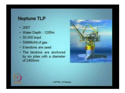
Neptune TLP 2007 constructed at 1300 meters approximately. So, all these are deep water platforms 50000 DOPD etcetera. The other kind of platforms is spar platform which is also having a similar response behavior to that of TLP, but of course, it is not a
