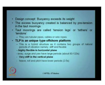
So, we will quickly browse through this design concept that is buoyancy exceeds its weight, we earlier discussed that. Weight is much lower than buoyancy, the excess buoyancy created is balanced by pretension in the taut moored cables, taut mooring or otherwise called as tension legs, because they are always in initial pretension. Generally these are tubular members or wire ropes TLP is any type of platform because it is having horizontal and vertical plane different behavior.
