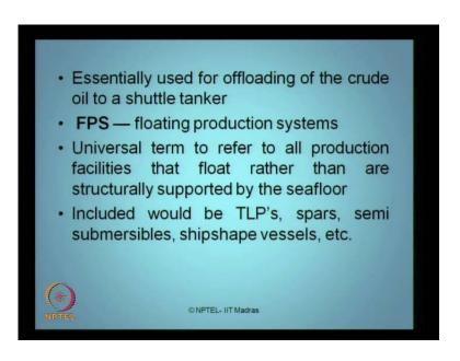
We just quickly go through this slide. It is not of very important to me, but still essentially used for offloading of crude oil to the shuttle tanker, FPS stands for floating production system whereas FPSO stands for floating production storage and offloading as well. So, in universal term being used, to be supported by the sea floor and included
