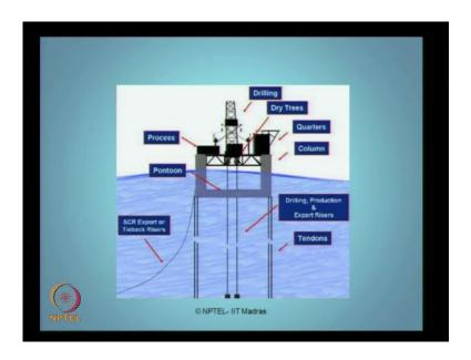
So, these are some of the components of a TLP, the drilling dry trees quarters, columns and pontoons and of course, the tendons.
