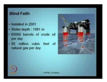
It is another important semi submersible constructed blind faith, installed in 2001 etcetera. It is a production platform. The next one is an FPSO which we all know, floating production storage and offloading.
