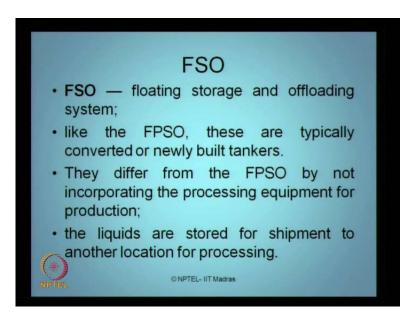
So, we will talk about FSO's also very briefly, floating storage and offloading. There is no production here production is on a different platform. It is associated with the production unit and FSO is also a kind of platform. They are actually existing tankers; I mean converted as floating structures which is essentially used for storage and offloading only, not for production.
