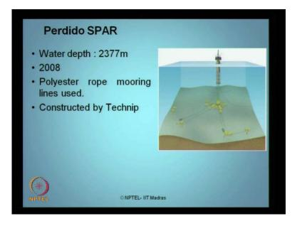
This is another spar platform what we have, Perdido spar. We can see the spread mooring system which can be seen in this photograph here. The advantage of this spar system is it goes deeper than TLP's because the cable or the tether cost is far relatively becoming inner springs in the system. It goes around 2300 meters, constructed in 2008, polyester rope mooring was used, constructed by the company naming Technip.
