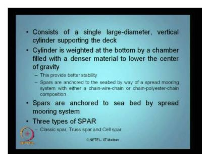
It consists of a single large diameter vertical cylinder which is supporting the deck, I will show you a photograph followed by this. The cylinder is weighed at the bottom by the chamber filled with denser material, that is how the spar is being installed. This provides better stability for the spar platform or the cylinder against lateral action of wind and waves, Spars are actually anchored to the sea bed by the way of spread mooring system.
