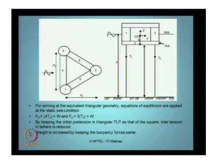
What is the basis for comparison is given here to arrive at a equivalent triangular geometry that of the square geometry there are two cases can be compared here by using the equations of equilibrium. In this problem, I can say the buoyancy can be 4 T plus W that is for square TLP because T naught is dimensional in each because the triangular TLP will be 2 T naught plus w where w is the weight of the platform by keeping the initial pretension same.
