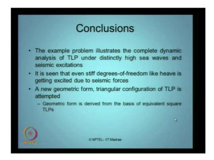
The example problem illustrates the complete dynamic analysis of TLP under distinctly high sea wave seismic excitations. We can see this from the example even the stiff degrees like heave is getting excited because of siesmic forces. Distinctly, a loop
