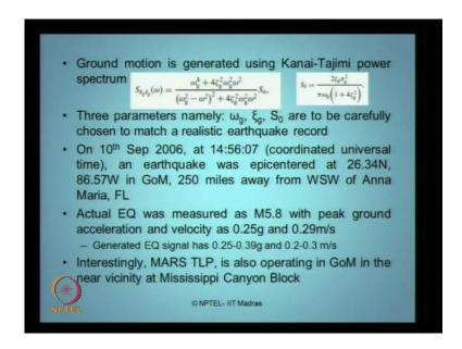
So, this is my Kanai Tajimi spectrum, we already had it it is an artificial using k p power spectrum there is the other one equation. There are three parameters of omega g zeta g s naught is the ground damping which is not the structural damping omega g is the ground structural damping and s naught is the spectral coordinator which is the problem which is available here.
