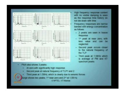
So, these are my power spectrum density of functions of heave pitch and sorry heave pitch and surge of course you can see this responses in the paper in detail. So, we will quickly look at the observations heave frequency response is no show visible damping. So, here it is not dying it is continuing here, there is no question of dying down heave response not dying down at all there is no visible damping present in this system which is computing for decay of response.
