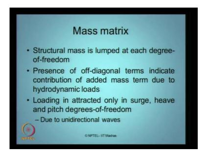
Mass term due to hydrodynamic loading the loading is attracted in this problem only in three degrees of freedom that is surge heave and pitch degree of freedom due to unidirectional waves structure. (Refer Slide Time: 25:58)
