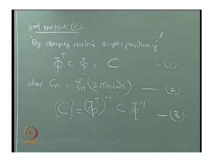
There is the third method we can do damping, this is by damping matrix super positioning, so I will do the super portioning with damping matrix and try to find the semantics of different matrix. So, we already know that phi transpose C phi is C where if you want to find C damping at the nth degree of or damping and we already know this is equal to zeta 2 m n w n for a classical damping. So, we know from this equation we can find C further as phi transpose inverse C phi inverse.
