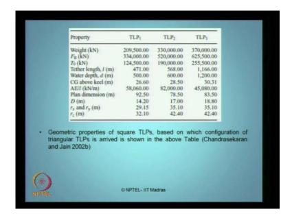
These are the properties of 1, 2 and 3, these are three different TLP's which are available in literature existing TLP's literature says that these are existing properties, so p equivalent triangular shape has been for TLP 1, TLP 2, TLP 3 is based.
