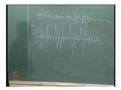
So, if you can pick up any one such process which can have realization of all the statistical parameters of the entire record, then that process can be said as ergodic process.
