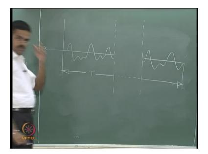
t is infinitely large. The record length is very very high. This is my x value, some preassigned value. Not 0 because we know sea surface elevation cannot be 0. This is my record, where this is my t. I said the cumulative distribution function will be given by the value of realization of x, which is less than or equal to x. I have a pre assigned value of x. So, I pick up those segments in the record, delta t 1.
