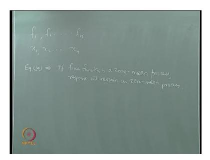
So, f y, f 1, f 2, f 3; f 1, f 2, etcetera or small n are realization of f of x. They are the set of team of f of x. Whereas, x 1, x 2, x n are realization of the response. So, connecting these two is the transfer function. So, we also see from equation 14, that equation 14 implies that, if the force function is a zero mean process, then response will also remain as zero mean process. So, let us quickly get the details of the response spectrum and see how does it look like.
