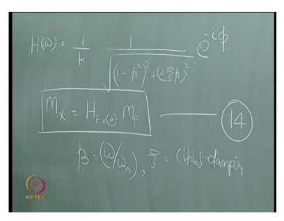
Based on which, we derived a simple relationship between the variance of the response to that of the variance of the force. But, here we are showing the corresponding connectivity between the mean value of the response and mean value of the force. And, we already know, in stochastic process, we are talking about realization of the force and the x value.
