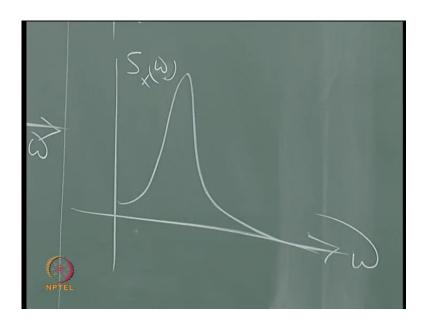
And, the response spectrum after connecting the transfer function to the load spectrum will look like this.
