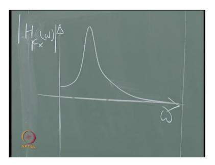
And, the transfer function, which connects this spectrum to the response will look like this; which I call H of F x omega absolute for different omegas of course. Basically, it will come to 0.
