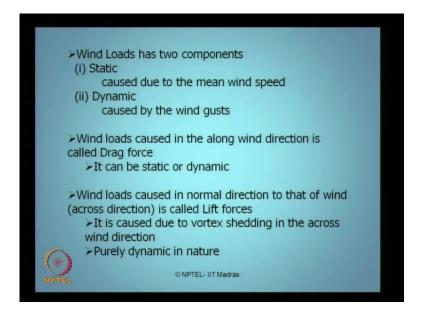
The wind loads along the wind direction is what we called as a drag drag force. They try to drag structure. The drag force can be either static or dynamic whereas wind loads caused in the direction normal to direction of wind, what we call across direction, is a lift
