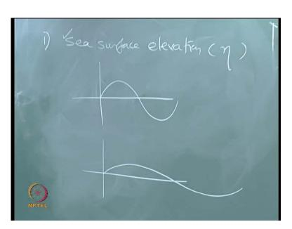
So, for a given wave force, I must first specify my sea surface elevation, which I call as eta, it is a standard notation. So, what do you understand by a sea surface profile? Many literatures say sea surface profile can be a sinusoidal variation; some literatures say. Look at the flat crest now; this tremendous variation given by people. So, the first confusion starts what to new elevation - sea surface elevation.?
