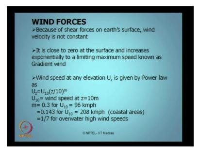
Look at the wind forces in general wind forces actually are caused because of the sheer force acting on the earth surface. Therefore, wind velocity does not remain constant it keeps on changing. So, let us quickly looked at the steps how do we worked out the wind force in brief because all of us have studied how to estimate wind forces in buildings or members on onshore. Now let us see how we can do it in the same principle or offshore structural movements?
