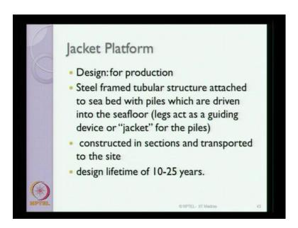
Jacket platforms are essentially production type platforms. It consists of steel framed tubeless structure, which is attached to the sea bed with piles. It is constructed in sections
