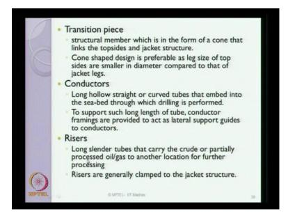
The transition piece is one of the important segments, a structural member, which is in the form of a cone, which connects the topside to the jacket structure. The jacket structure is nothing but the leg; topside is nothing but the details of the machineries, what you saw on in the last slide. The topside and the jacket are interconnected by a piece, which is conical in shape, which rocks the deck to that of the legs.
