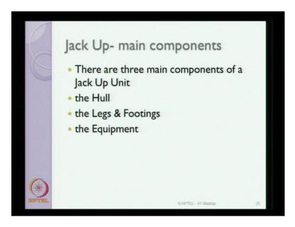
We have already seen, some of the components of jack up rigs. Let us quickly see the main components of a jack up rig. Essentially jack up platforms consists of three main components. The hull on which the whole mechanical devices are equipped the legs and the footing on which the hull rests of course, the equipments which are used for drilling and production.
