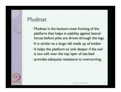
Mud mat is one of the vital component of this kind of structure, which is a bottom most frame of the platform, which helps in improving stability against lateral forces. Before the piles are driven through the legs. It is similar to a large raft made out of timber; it helps the platform to sink deeper. If the soil is too soft, it provides adequate resistance against over turning in case of any installation problems.
