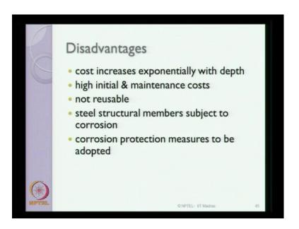
There are some disadvantages of these kinds of marine structures, the cost of these structures increase exponentially with increase in water depth. They have very high initial and maintenance costs, they are not mostly reusable. The steel structural members are subjected to extensive corrosion in the sea environment. Therefore, corrosion protection measures become very important and they are also expensive.
