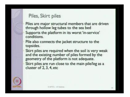
If you look at the piles and the skirt piles is a vital components, on which the jacket structures rest. Piles are major structural members that are driven through hollow leg tubes to the seabed. It supports the platform in service condition; piles also connect the jacket structures with the topsides. Skirt piles are especially required to improve the lateral stability of the platform. When the soil is very weak, skirt piles are generally done in groups of two, three and four etc.
