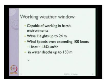
If you look at the working weather window of this kind of platform they are capable of of course working in harsh environment, the wave height is up to 24 meters can be allowed in this kind of operation. The wind speeds even exceeding 100 knots can also be sustained by this kind of platform. Ladies and gentlemen one knot is about 1.85 kilometer in hour. They are successful in operating up to water depths of one fifty meters.
