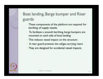
If you look at the boat landing, barge bumpers and riser guards; these are also ancillary components of the platform, which are required for berthing of the supply vessels. To facilitate a smooth berthing, barge bumpers are installed on each side of the boat landing. This reduces the vessel impact on the jacket structure; the riser guard also protects the oil
