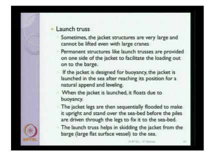
Launch truss, is one of the vital components, sometimes when the jacket structures are very large in size and cannot be lifted even with large cranes they are done. The permanent structures like launch trusses will be provided on one side with jacket to facilitate the loading out on the jacket to barge.
