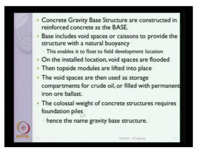
Concrete gravity base structures are constructed with the reinforced concrete as the BASE. The BASE includes void spaces; otherwise, what we call them as caissons. They are essentially used to provide the structure with natural buoyancy. This enables the structure to float to the field development location, when they are void or when they are empty. Once they reach the installation side, these void spaces are flooded with water.
