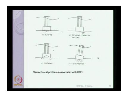
There are some specific geotechnical problems associated with gravity based structures. What you see the slide are four special critical problems that are closely associated with any massive type of structure, which are founded in sea bed. Sliding is a problem associated, which has lower resistance to lateral load upon the wave or wind load on gravity base structure.
