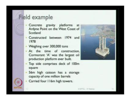
Looking at the field example one can see this interesting field example, which is a concrete gravity placed platform, which is constructed at Ardyne point on the west coast of Scotland. As you can see, these are the towers resting on the caissons, which are twenty four in numbers, which are very massive in size; these platforms are constructed between 1974 to 1978.
