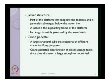
The jacket structure essentially consists of part of the platform, which supports the topside and generally it is submerged below the water. A jacket is a supporting frame of the platform, which is mainly designed to resist the wave loads acting on the platform. Crane pedestal is a large structural tube that supports the offshore crane for lifting purposes. Crane pedestals function also as diesel storage tanks. Since the diameter is large enough to house fuel.
