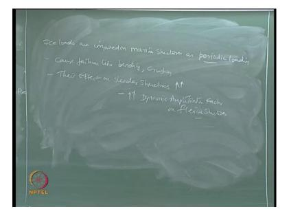
Therefore, ice loads are impost on marine structures, as periodic load. They can cause failures, like bending, crushing, and their effect on slender structures, is very high. It means, this increases the dynamic amplification factor, on f is say flexible structures. More interestingly, to quantify the ice load people have done the search, how the ice load can be quantified. While they did this work, they founded very important parameter, which governs the ice load.
