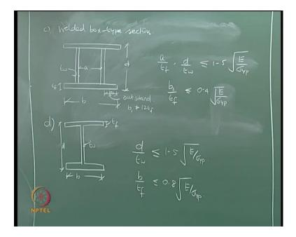
Now, you also have welded box sections, these are common; these are actually used for pipe racks in marine structures. People construct the box section and insert the pipes, coned insert this and welded box types are very interesting section like this, you have upper and lower flinch plates then with that flinch plates you create a box section. This a typical welded box type section, this is what we call technically an outstand and let say this is my breadth of the section.
