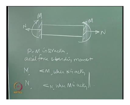
So, you must agree that if you got a beam simply supported beam for a span of l, let us say I have a fixed beam. I have fixed beam of span l subjected to moment subjected to n movement as well as axial force. I can call this as M and this as N there will be of course, a variation between this ends. Let us say the moment and actual force acting you will see that the P-M interaction that is the interaction between the axial force and the
