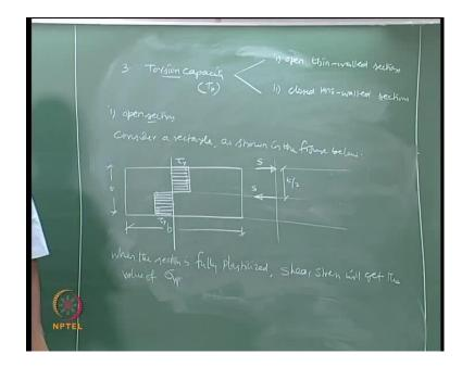
So, we now estimate the torsion capacity we estimated the axial capacity, we estimated the shear capacity, we will now talk about torsion capacity. So, we divide this into 2 level of understanding, 1 is open thin walled sections. I will come to the point what are thin walled sections, second is closed thin walled sections. The name itself very clearly tells, what is thin walled section.
