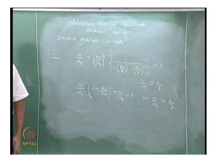
So, we discussed for the I section, the combined axial loading under bending moment and axial force. Let us say p N interaction, we said that M by M p plus N by N p square. This is one kind of interaction diagram where, the value of N by N p is lower than the capacity of the web. Alternatively its true interaction for N by N p greater than or equal to A w by A.
