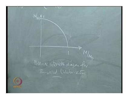
This the B M N interaction diagram, for thin walled tubular sections. Now, we will talk about some of the concepts of impact analysis.
