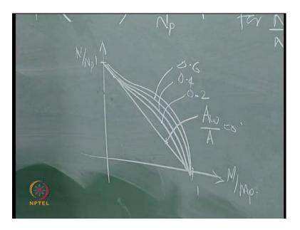
And we already saw that interactions diagrams for M by M p versus N by N p at 1 and 1 for A w by A ratio becoming 0. This becomes a linear line then this keeps on varying for different ratios of this curve is for A w by A is 0, and of course this is for 0.2, 0.4 and 0.6 and so and so on.
