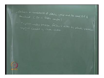
So, the failure a combination of plastic yield and the stability of the chord therefore, we can say it is highly complex, where as in T joints in the tension failure is either by plastic yield, or rupture caused by shear stress. So, here the chord gets separated at these junctions.
