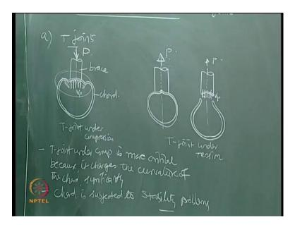
So,I am drawing it here separatelyand to oppose this,there will be shear stress and in this case to oppose this,there will be shear force. So, the chord will get disassociated or the curvature of the chord changes significantly to the dotted line and then subjected to shear
