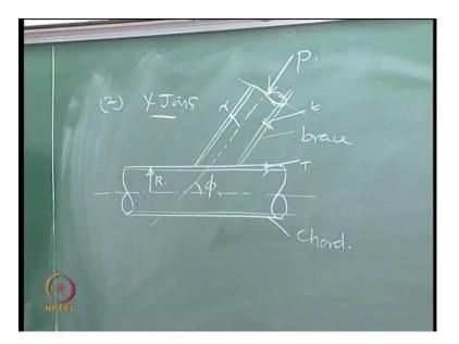
Let us talk about ultimate strength capacity of Y joints.Y joints can also be again in tension and compression depending upon what is the load applied on the braceis the typical Y joint.This is what we call as a brace,this is what we call as chord,this is mythickness of the chord,the radius of the chord as this thickness of the brace,this is I say small t. This is I say capital T, this is I say small r and this angle is phi.So, let us say this subjected to compression or tension,let us say P.
