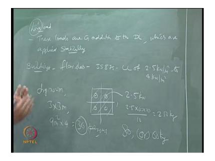
Next of course, will be the Live load, these loads are in addition to to the dead load, which are applied statically, remember this. So, static component you may say sir live load will
