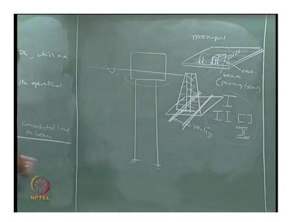
Let us say I have an offshore platform may be a TLP;may be a jacket top more. Now, I pick up only thisand try to draw, I call this as a deck supporting system. So, the deck comprises of essentially, a plate. I am just drawing only a line diagram. Essentially a plate
