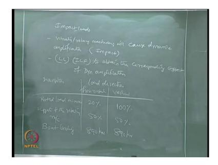
Say Impact loadswe all understand that any Vibratingor Rotary machinerywillcaused dynamic amplification, which I caused as impact. Therefore, Live loads are multiplied by Impact loads factor to get the corresponding effect of dynamic amplification, you understand this. Just to get the amplification of the dynamic effect on the members, we multiply the live loads which some impact factors that is why we call this Impact factors on the Live loads Impact load factors, so again a table.
