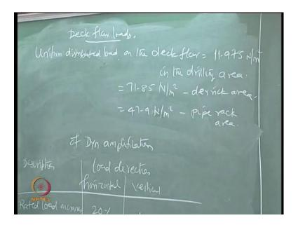
In addition to this, what would be the common uniform distributed load which is advised on the decks, this is 11.975Newtonper square meter in the drilling areathese are all original Live loads, 71.85Newton per square meter in the Derrick area 47.9Newton per square meter in the pipe rack area, these are what we called asdeck flow loads, these are all the loads which comes on the decks flow.
