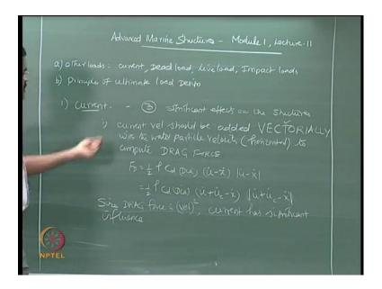
So, let us talk about the effect of current or the influence of current as a loadon marine structures. Current has a actually three significant effects on the structures. Let say for example, the first could be current velocity should be added vectorially with the water
