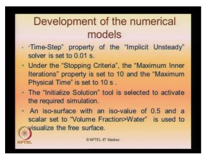
The "Time-Step" property of the "Implicit Unsteady" solver is set to 0.01 seconds. Under the "Stopping Criteria", the "Maximum Inner Iterations" is set to 10 and the "Maximum Physical Time" is set to 10 seconds. The "Initialize Solution" tool is selected to activate the required simulation. An iso-surface with an iso-value of 0.5 and the scalar set to "Volume Fraction greater than Water" is used to visualize the free surface.
