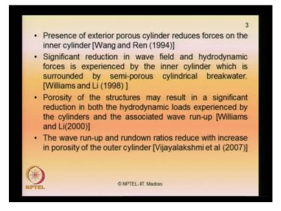
Presence of exterior porous cylinder reduces force in inner cylinder; this has been ascertained and verified by Wang and Ren. Whenever you have got an outer cover which is porous, over and inner cover or inner cylinder which is solid, there is a force reduction on the inner cylinder, I am talking about reduction on the inner cylinder. This has been verified and quantified by Wang and Ren.
