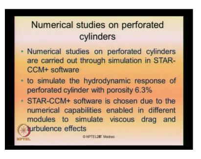
Subsequently this has been also verified using numerical studies. The numerical studies perforated cylinders are carried out using a software simulation in star CCM. Now idea was to simulate that hydrodynamic response with the porosity of 6.3 percent, softer CCM is chosen because the numerical capabilities enabled in different modules to simulate viscous drag and turbulence effects are good in this software.
