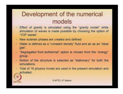
The effect of gravity is simulated using the gravity model while simulation of waves is made possible under the option of VOF waves. The new eulerian phases are created and defined, water is defined as constant density fluid and air as an ideal gas. The "segregated fluid isothermal" option is used for the energy group. Motion of the structure is selected as the stationary for both the simulations. Total of 16 physics models are used in the present simulation and then activated subsequently.
