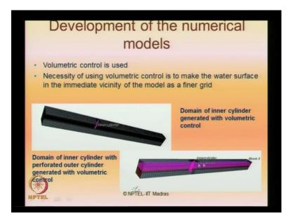
This is how the model looks like for a domain of inner cylinder and the domain of inner cylinder with perforated outer cover, this is a domain what we are showing.
