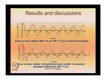
The results and discussions as you see here for force on inner cylinder in numerical simulation and force on inner cylinder with perforated outer cover in the numerical simulation, for the same wave period and wave height.
