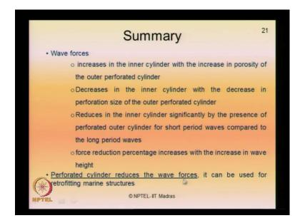
So we can see that the wave forces increases in inner cylinder with increase in porosity, decreases in inner cylinder with decrease in perforated size, reduces in inner cylinders significantly by the presence of perforated outer cylinder for a short period waves compared to long period waves. Force percentage reduction increases with increase in wave height, so perforated cylinder reduces wave forces which can be seen as one of the direct method of retrofitting marine structures.
