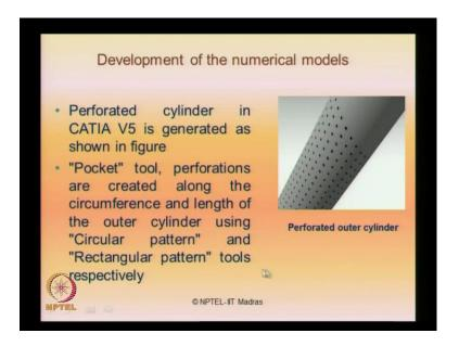
The numerical model of a perforated cylinder is developed in CATIA V5 as shown in the figure here. The pocket tool perforations are created along the circumference and the length of auto cylinders using circular pattern and rectangular pattern tools respectively.
