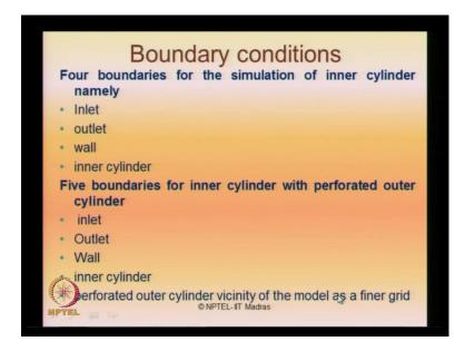
Different boundary conditions deployed for the analysis for the inner cylinder is basically inlet, outlet, wall and of course the cylinder, whereas by perforated outer cover we have got 5 boundaries inlet, outlet, wall, inner cylinder and perforated outer cylinder vicinity of the model as the finer grid.
