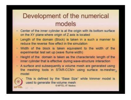
Let us quicklysee some of the details of the numerical models; the centre of the inner cylinder is kept as an origin because bottom surface in x y plane, the length of the domain block is taken in such a manner to reduce the reverse flow effect in the simulation, the width of the block is taken equivalent to the width of the flow, the height of the domain is taken equal to the characteristics length of the inner cylinder that is
