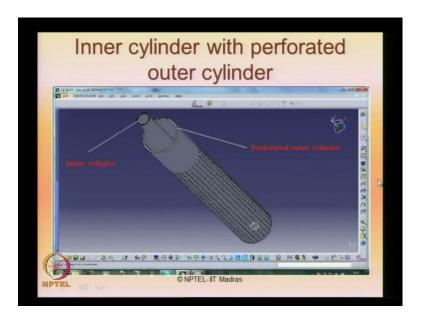
This picture shows you the inner cylinder with the outer perforated cover generated in star CCM for numerical analyses.
