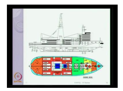
This is a classical topside view of a typical navigation ship, which has been converted to a drill ship can see here. There are two classical large moon pools, which are centrally located on the deck through which the drilling operation generally takes place. Many can see the other complexities or other details are similar to that of any typical navigation vessel as you see in case of a ship.
