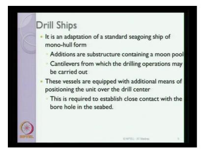
Drill ships, ladies and gentlemen is nothing, but an adaptation of a standard seagoing vessel which comprises of a mono hull form. There are some additions done in the substructure, which contains a moon pool, which enables the drilling to take place. There are cantilevers attached to the seagoing vessel from which the drilling operation can be also carried out in conjunction with that of the moon pool.
