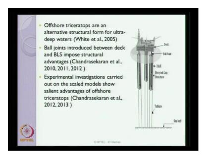
The picture what you see here is the conceptual study extended for deep water platforms, which is called triceratops by white et al in 2005. This is suggested as an alternative structural form for ultra deep waters. Essentially, triceratops has a deck and a hull, which are connected by means of what we call as ball joints. Hulls are nothing, but the buoyant leg structures, which are anchored to the seabed using tethers as similar to that of tensional platforms.
