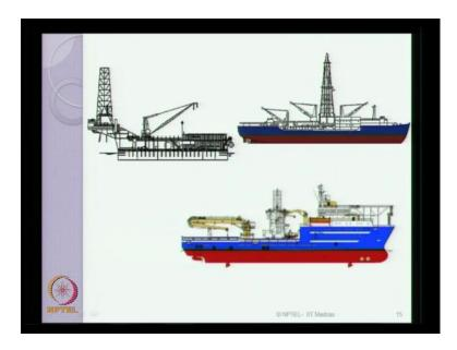
These are some of the views and photographs of a typical drill ship, which consists of all the essential features of classical topside of any platform, which can equip or which can perform drilling operation. It has got a derrick mask it has got cranes for performing different operations, it has got the flare boom the living quarters and all mechanical topside complexities as desired in case of any production platform, which is meant for deep water drill.
