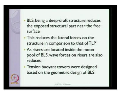
BLS, being a deep draft structure reduces the exposed structural part near the free surface. This reduces essentially the lateral forces acting on the members in comparison to that of tensional platforms. As risers are located inside the moon pool of BLS wave forces on risers are significantly reduced which advantage of these kinds of structures. Tension buoyant towers were designed based on the geometric design of buoyant leg structures.
