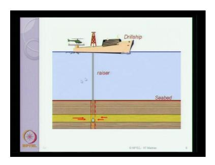
The conceptual figure shows here. How the risers are also connected to the drill ship, while the drill ships is in operation. As I told you, it is very important that the dynamic positioning system should keep the drill ship enable in such a way that the motion controlled is happened, as per the desired value, so that the risers and the drill strings are not disconnected from the drill ship when the drill ship is performing the drilling operation.
