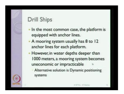
In the most common case of a drill ship the platform is generally equipped with the anchor lines. A mooring system comprising these anchors usually has 8 to 12 anchor lines for each platform. However, in water depths greater than 1000 meters a mooring system becomes highly uneconomical and impractical therefore, people generally deploy dynamic positioning systems for using drill ships in deeper waters practically more than 1000 meters.
