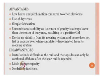
It has got many merit is and demerit is low heave and pitch motion compared to other platforms use of dry trees simple fabrication and unconditional stability because CG is much higher than the geometric center or the center of buoyancy derive no stability from mooring system.
