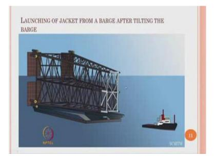
This picture gives you again a view of how a jacket is launched, using the barge after titling the barge this is actually the d which is storing and launching once the launching is completed it be upended and the platform become the jacket becomes vertical and these are the spud cans or the portions where connected to the pile foundation at the sea floor.
