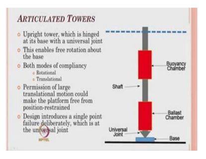
The second type of platform which is also compliant in nature, which has got merit is better than the guyed tower is articulated platforms the term articulation refers to an universal joint, which is again similar to the that of a ball joint this shows a single unique tower which is connected to the buoyancy chamber, and the ballast chamber ballast chamber at the bottom and buoyancy chamber closer to the mean sea level which is interconnected to the central tower.
