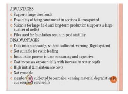
Therefore, the platform is able to have good stiff arrangement as it can alleviate the lateral loads acting on them. There are some demerit is of this platform the platform will fail instantaneously without sufficient warning, because that is a general behavior of any rigid or brittle system, this is a platform is generally not suitable for cyclic loading.
