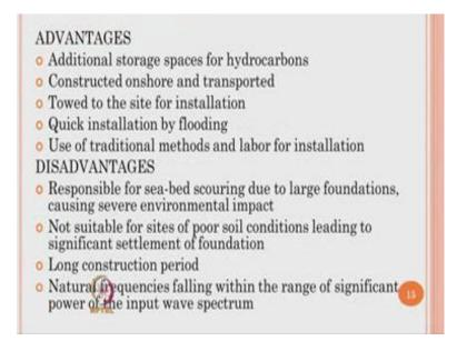
These platforms have couple of merit is and demerit is let us quickly see them the merit is could be the following it has got additional storage space for hydrocarbons. Constructed onshore and they can be transported in modules, towed to the site for installation, quick installation is possible by a mechanism called flooding. Use of traditional methods and labor for installation is making this platform time of installation as minimum as possible.
