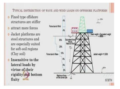
Let us quickly look at a typical distribution of wave and wind loads on a given offshore platform which is fixed to the sea bed. The fixed type offshore structures become stiffer because of a simple reason the whole template structure is being anchored firmly to the sea bed. When they are anchored firmly to the sea bed through pile foundations then, the movement of this particular structural system under the lateral forces is highly restricted.
