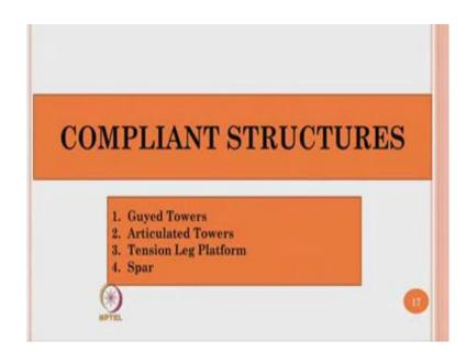
The second type of offshore platforms is what we call as compliant structures the variety of compliant structures, can be the following guyed towers articulated towers tension leg platforms and spar platforms.
