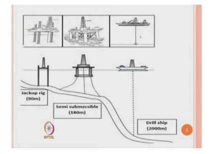
This figure shows you the conception understanding of what kind platform can be deployed floating type can be d deployed at different water depths up to 90 or save 100 meters one can go for jack up rigs beyond 100 meters one is comfortable with semi submersible up to about 200 meters and beyond 200 or 250 meters prefer to take a drill ship which can also be capable of exploratory drilling up to depth of as deep as 2000 meters.
