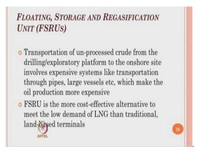
The other kind of offshore platform which is again the new generation platform is a floating, storage, re-gasification unit.
