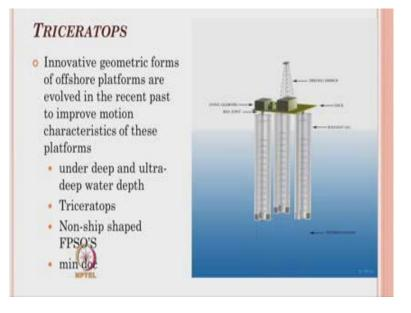
The second verity of structure what you see here which is new generation platform is offshore triceratops. The word triceratops indicates there are three pairs of buoyant leg systems. These are buoyant legs which are not interconnected, which are of course anchored to the sea belt using tethers or tendence as in the case of a TLP.
