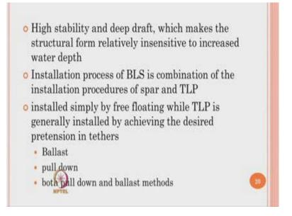
High stability and deep draft makes these platforms in sensitive for increase water depth. Installation process of BLS is a combination of installation procedure of spar and TLP. They install simply by free floating, while TLP is generally installed by achieving the desire pretension in tethers either by ballasting or pulling down or both pull down of tethers and ballast methods.
