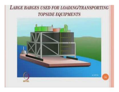
Large barges are also used for loading transporting top side equipments, because you know modular construction is enabled in offshore platform design.
