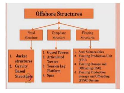
Just to have continuity offshore structures are essentially divided into three categories; fixed structure, complaint structure and floating structures. Fixed structures have got two verities within them; jacket structures and template structures, gravity based structures or GBS platforms. Complaint structures have four verity within them; guyed towers, articulated towers, tension leg platform and spar platforms.
