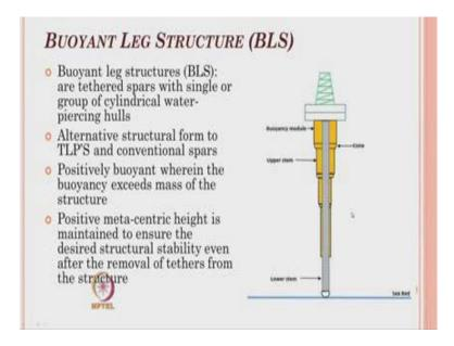
Top on the list in the new generation platform is Buoyant Leg Structure, abbreviated briefly as BLS. A typical tower or stem is connected to the sea bed using a spect scan or a universal joint similar to that of previous kind of an offshore platform. Now the interesting part of this particular type of platform is that there are different buoyancy modules attached to the central tower at different locations so that the buoyancy can be adjusted depending upon sea state.
