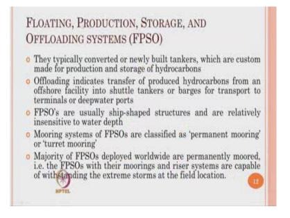
The next variety is floating by nature of geometry, production, storage and offloading by nature of its function is called FPSO. They typically or actually converted type tankers which are custom made for production and storage of hydrocarbons. The essential function of an FPSO is a storage capacity which is not otherwise seen in normal conventional platforms meant for exported type.
