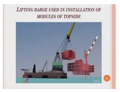
Lifting barge is one of the common facility being used for installation and commissioning during essentially during the top side installation what we call as a (Refer Time: 30:08).
