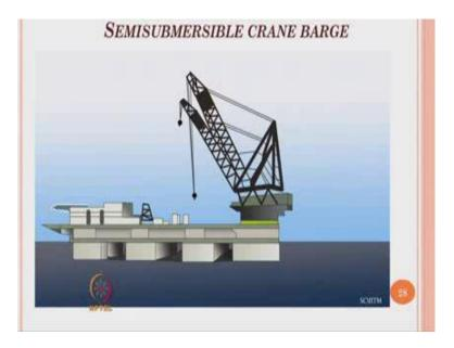
The photograph what you see here is semisubmersible crane barge. Now we can understand very clearly that a platform which is not tankered to the sea bed or connected a sea bed using piles that is semisubmersible needs a crane barge which is used for uploading or transferring oil from one vessel to the another vessel or shuttle tanker.
