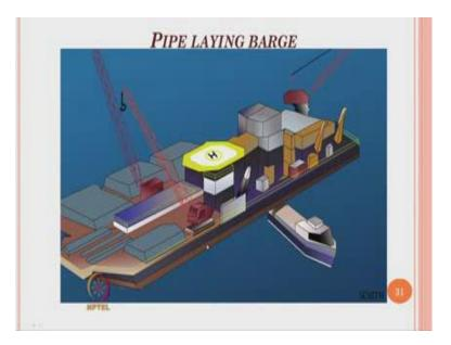
Pipe laying barge is another kind of large floating vessel which essentially used for lying of pipes. Pipes can be used for transporting oil from offshore to onshore locations.
