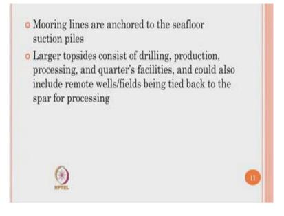
The mooring lines are anchored to the seafloor using piles, which is a suction type pile. Larger top side consist of drilling, production, processing, living quarters, and go also include remote well fields being tied back to the spar for processing.
