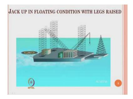
When a jack up is in a floating condition this how it looks like all the tower like system or the (Refer Time: 08:09) type towers will be kept above the deck and only the deck will made to float like a simple sea going vessel on reaching the site in location the deck will be jacked up. So, that these legs will be pulled down they will connected to the sea floor using the spec scan system as you saw in the case of a simple arcaded towers.
