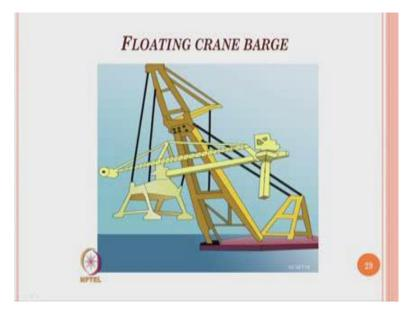
This picture shows floating crane barge which by itself floats and can be moved from one location to another location as the system demanded.
