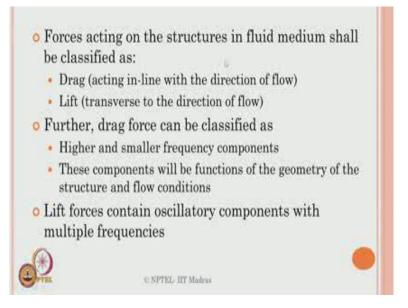
Therefore forces acting on the structures in the fluid medium shall be classified as 2 one is a drag and the lift forces. Drag is what we call in line force acting in the direction of
