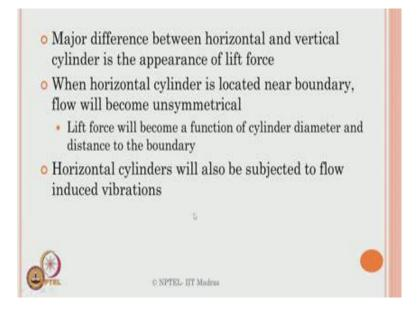
Which result in major difference between the horizontal and vertical cylinder is the appearance of lift force. When the horizontal cylinder is located near the boundary flow will become unsymmetric. Lift forces will become a function of cylinder diameter, and distance to that of the boundary from the axis of the member horizontal cylinders will also be subjected to flow induced vibrations which will cause secondary oscillation to the given system.
