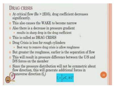
There is something called drag crisis in the literature which is very important for drag dominant structures in offshore platforms. At critical flow for example, the Reynolds number exceeds 2 e power 5, then the drag coefficient decreases phenomenally. This also causes a wake to become very narrow.
