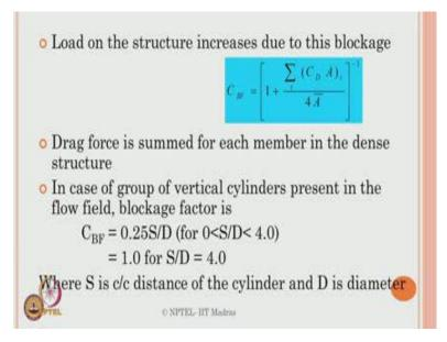
Now, let us coming back to the point or the load on the structure increases due to this blockage effect which is given by this equation where C BF is given by the blockage factor. Which is given by this equation are in case of group of vertical cylinders present in the flow filed you can also calculate C BF using this relationship where s is a center distance of the cylinder, and where d is the diameter of the cylinder.
