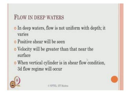
When we move on to shallow medium to deep waters, then the flow field slightly gets altered. In deep waters the flow is not uniform with the depth. It varies. We all know that because a water body is velocity in acceleration, keeps on challenging with respect to depth. It is maximum at the mean sea. And it is practically 0 when it goes through the sea bed.
