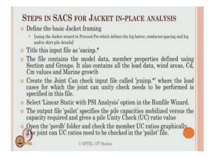
Let us quickly see what are those steps in a jacket modeling in sacs in general for inplace analysis define the basic jacket framing use the jacket wizard in precede pro in sacs module which defines, the leg batter, the conductor spacing and leg and a skirt file details title. This fire as an input as INP dot star, the file contains the model data, the member property is the C d C m value, the wind area and the low data marine growth etcetera.
