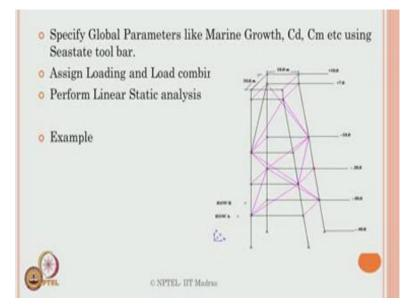
Then a typical result is available as an example here, jacket has been created with the r l of minus 42 plus 10 about 50 meter rho and rho b are the 2 rho's of piles available or the
