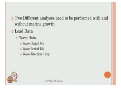
The load data is be used as wave data significant wave height 8 meter and wave period 12 seconds and wave direction is 0.
