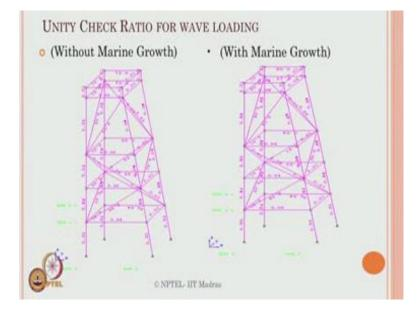
Then unitary check with and without marine growth is been done. And you will see for example, look at the specific member; this member is a having the number of 0.04 is an unitary check it is safe it means the number does not exceed one it is safe. We can check
