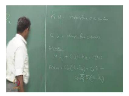
Now, interestingly let us look at some terminology; let us say K u. Let say C u dot. Now, u being the displacement of the structure, K u will be the restoring force which is stiffness proportional of the structure - u naught b, the damping force which arise from the structure, so structural damping, not the hydro dynamic part; because u dot has been taken, where u is the displacement of the structure.
