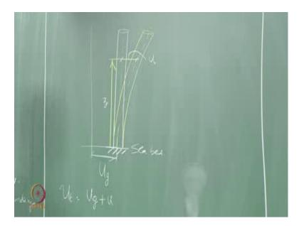
So, if you have a cylinder whose initial position is vertical, which is fixed to the sea bed and hollow cylinder, when the displacement for the ground or the sea bed is given, the cylinder being a cantilever stack will bend.
