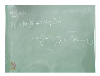
So, let us write the equation of motion. Now, the given system; combining all these terms, I should say the mass moment of inertia will have two terms; theta double dot. I am using a classical damping; not really a damping. plus, K of one plus r t of theta should be equal to; let say equation number one. That is the equation of motion now.
