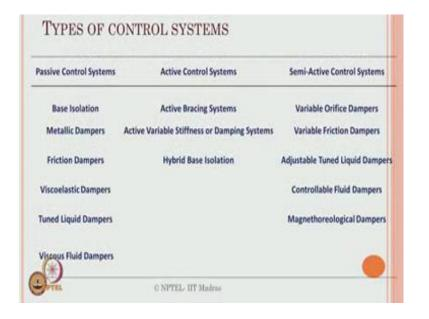
So, let us see the type of control system here, passive control are listed as base isolation metallic dampers friction dampers, viscoelastic dampers, tuned liquid dampers called as TLDs and viscous fluid dampers. Active control systems are active bracing systems,
