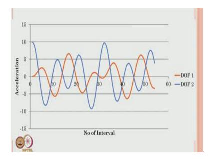
This is how you get the time variation of the displacement, velocity and acceleration using a numeric integration scheme as suggested by Newmark in 1960 s.
