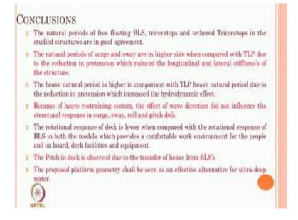
The natural periods of the free floating BLS triceratops and tethered are in good agreement this is one of them with that of the experiments. The natural periods of surge and sway are higher compared to that of TLP making it reduce in pretension in tethers.
