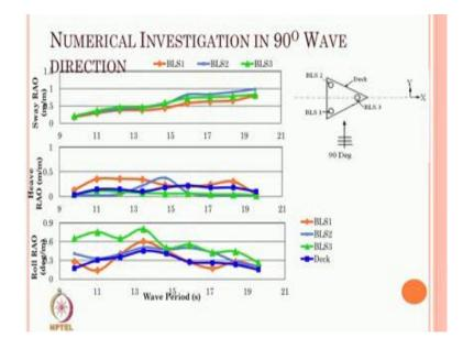
So, it shows that the deck and the heave of one of the BLS may be BLS 1 2 or 3 as shown in the common literature exactly behave monolithic or integrally connected between the deck and BLS as such for all degrees of freedom action; 180 degrees as well, and so on.
