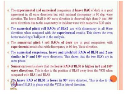
The numerical picture of BLS 2 is a discrepancy because of the wave direction effects. The heave of heave RAO of BLS 3 is much lower 90 degree because BLS 3 is the one which is far away the wave approach angle. Therefore, this is not influenced by the wave direction because the vertical center of gravity in the later direction is shifted.
