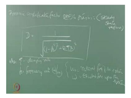
Now, let us compare this with the classical dynamic amplification factor is given by, this is of course, for a steady state response which is given by 1 by root of 1 minus beta square plus 2 zeta beta square where zeta is the damping ratio, and beta is the frequency ratio, which is omega by omega n where omega n is a natural frequency of the system. And omega is excitation frequency applied upon the system, this already we know is an established relationship we know this, just derive this.
