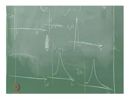
If you know the input spectrum maybe, whatever may be the spectrum I will get my output spectrum response spectrum using a connectivity which is m x the mean value of the response can be given by the transfer function mean, value of the force we already know this.
