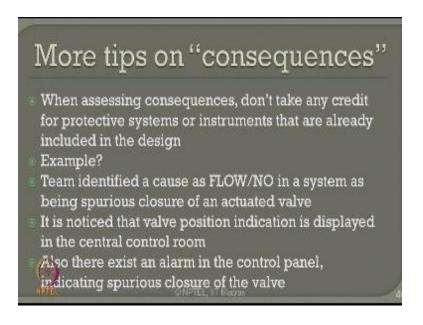
Also there came in alarm existing control panel which will indicate the closure of this valve, these are all already present in the design system do not try to take an advantage of this and do not try to over wrote these while writing the consequences in a given report.
