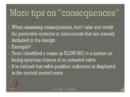
I can show an example the team identified a cause as flow or no in a given system as being spurious closure of an actuated valve it is notice that the wall position indication he displayed the central control room one can imagine that the central control room has an indication of a closed equation of the wall that is a safeguard in the design, do not try to assume that since this is available consequences cannot occur.
