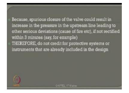
Because the spurious closure of the valve could result in increase in pressure in the up streamline which leads to see these deviations can result in fire if not rectified within few minutes for example it can cause explosion, therefore do not credit for productive systems or instruments that are already in place which included in the design in your consequences column of the report.
