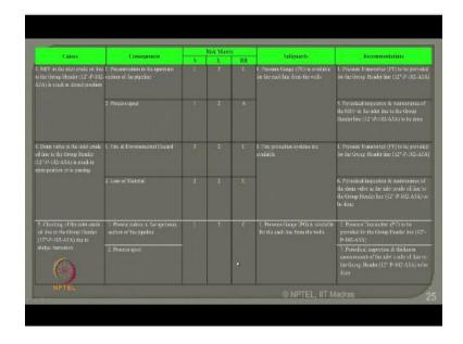
The non return value in the inlet crude oil can also fail if there is a case the pressurization will happen which will cause risk ranking as C of course the pressure gauge is available to check the functionality of the non return value. However, we also recommend pressure transmitter to be provided in the line to check any failure of non return value. Similarly one can look at all these numbers automatically done please understand interestingly.
