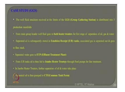
Where oil gas and water together are connected from here the y oil goes to emulsion receipt tank where as gas is flared of and water is going to a fluent it in plant subsequently oil from emulsion receipt tank goes to Jumbo heater Treater where this further treatment and the water goes has a steam of there is oil is in taken separately and fed and stored into CTF this is called common tank form now let us see the process instrumentation diagram of this.
