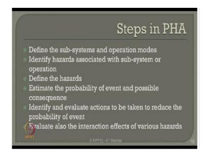
Now what are the steps involved in canning about preliminary hazard analysis? You have to define the sub system and the operational modes of the plant, one should identify hazards associated with a sub system or operations, define the hazards very clearly that arise during the process, estimate the probability of events and possible consequences that arise from these events, and therefore finally identify and evaluate actions.
