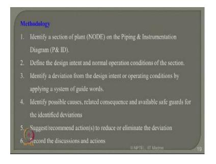
Let us quickly explain very briefly the methodology used for process in a group gathering station. Now the methodology of HAZOP report follow step by step in a given process piping and instrumentation diagram first let us identify the section of the plant which we call as node of the plant. Friends please understand HAZOP report is never done for the entire plant it is then only for segment ways of the plant.
