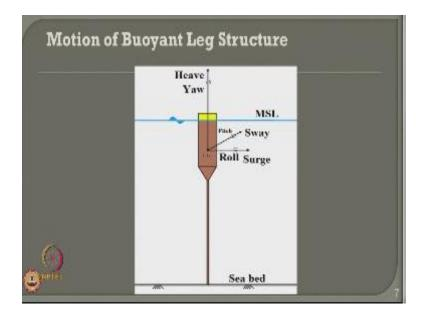
Let us now quickly see what are the motion characteristics of a Buoyant structure alone the buoyant structure has got essentially six degrees of freedom as any floating body has such way and row heave or the translational motions roll pitch and yaw or the rotational motions with respect to any specific degrees of freedom namely x axis y and z axis respectively the buoyant structure which is a deep draught element which will be anchored to the seabed using a tapered leg or a strained leg.
