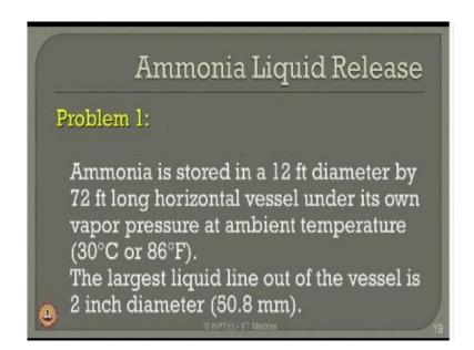
Let us say ammonia store in a 12 feet diameter of a 75 feet long horizontal vessels under its own vapor pressure at ambient temperature are about let us say 30 degree Celsius the largest liquid line which is extracting out from the vessel is about 2 inch in diameter which is 50.8 mm.
