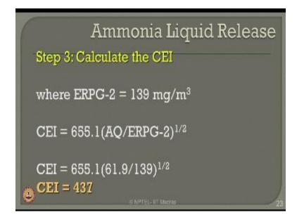
Once you know this I can now directly compute the chemical exposure index number but chemical exposure index number is relevant to detail difference of ERPG values for ammonia from the chemical engineering handbook one can find the ERPG 2 concentration is 139 mg/m<sup>3</sup> therefore CEI will be nothing but the equation as 655.1 x AQ/ERPG -2 <sup>1/2</sup> if is substitute the values because AQ is 61.9 which it got from the last slide.
