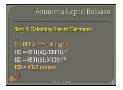
Let us see for ERPG 2 of 139 milli gram per cubic meter Hazard distance given to this equation I substitute the values I get the rod distance in 4372 meters on the other hand up to 4.372 kilometers if ammonia liquid is discharged from this vessel at a boiling temperature off so ands so then it will not cause irreversible effect on human being because ERPG dual concentration team says on states that it should not cause irreversible effect on human organism.
