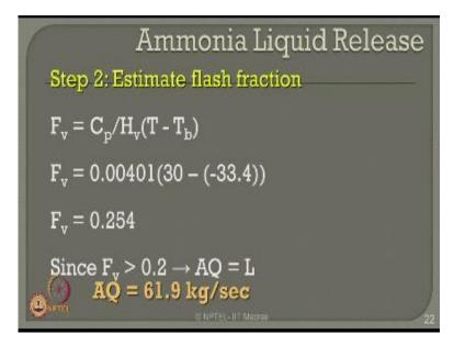
Then airborne quantity is completely assumed to be the liquid since then this value FV exceeds 0.2 that is 0.254 then the airborne quantity will be exactly equal to the value of L which we computed from the last slide, therefore airborne quantity now will be 6 1.9 kg per second which is computed from the last equation.
