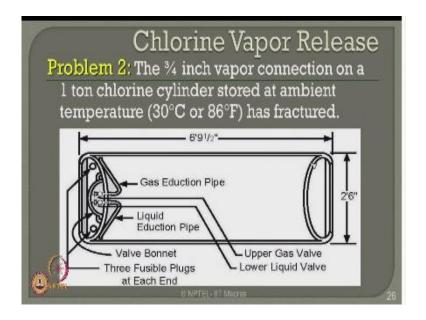
Let us take up another example which the chlorine vapor release, the first example problem was on ammonia liquid release. Now I am working a problem on chlorine vapor release let us say I have an object or a vessel which has got a gas ejection pipe we are having a liquid ejection pipe is a valve bullet which controls the chlorine vapor release completely there are three fusible plugs at each end of this container.
