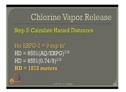
Now I want to compute directly the CEI the ERPG level 2 for clearance vapor is 9 mg cubic meter I substitute the value I get CEI as 188 then I compute a hard distance ERPG 2 I get the hard distance as 1.878 km.
