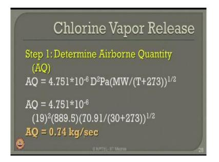
Step one determine airborne quantity of the square invertors given by this equation I know the values substitute them I am converting them into Kelvin's substitute them I am adding to 73 here substitute them and get along quantity as 0.74 kg per second.
