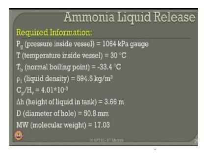
Now the required information to be chemical exposure index or chemical risk analysis of the following, one must know what is the pressure inside the vessel which is a given data which is 160 1064 kilo Pascal gauge pressure the temperature inside the vessel as we read from the problem is 30degree Celsius, the normal boiling point of ammonia liquid is minus 33.4 degree Celsius taken from the chemical engineering handbook.
