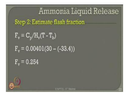
Which is CP/HV (T-Tb) boiling temperature Fv is now obtained by substituting the values of the equation and we know the operational temperature is specific problem is 30 degree Celsius and the boiling point of ammonia taken from chemical engineer handbook is minus 33.4 therefore the volume of flash fraction in the specific problem comes to be 0.254, now if this value exceeds 0.Q 0.2.
