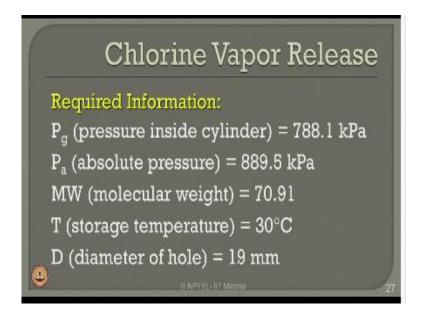
Let us see what are the required information for solving this problem, pressure inside the vessel 788.1 kilo pascal which is given in the problem with the gauge pressure the absolute pressure is of course 899.5 kilo pascal molecular weight of chlorine vapor is 17.91 the temperature of storage is 30 degree Celsius given in the problem diameter of hole is  $3/4^{\text{th}}$  inch which is about 19mm.
