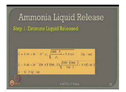
The liquid release can be given by a simple expression as shown here substitute the values of the diameter D 50.8 density which is given gage pressure is available to me delta h is the height of the liquid column of the ammonia being stored in the vessel which is 3.66 meter, so all of them are unit compatible therefore if you substitute them in respective units then I will get L which is the liquid released ammonia in kg per second. For this problem 61.9 kg per second.
