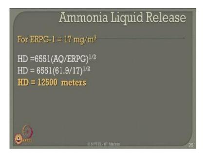
Will be 12.5 km so it is very evident for upto 12.5 kilometers if you stay beyond 4.375 kilometers that is from 2 level to 1 level you will not even get objectionable to wither, on the other hand if you are staying beyond 10.5 kilometers will have no effect of this liquid released in airborne contain apart on the societal risk.
