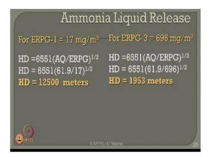
For ERPG 3 which is the little concentration which is very high 696 milligram per cubic meter the hazard distance comes to be 1.953 kilometers. So if you are staying less than 1.5 kilometers from the plant where the liquid is released or discharged as a given rate then this show that you will have a reversible effect in your body which may end up in fatal also.
