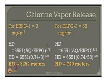
For ERPG 2 you can also do this for ERPG 1 and ERPG 3 which gives me the respective values shown on the screen. So ERPG 3 is as close as 0.75 kilometers from the plant source whereas ERPG 1 is as far as 3.254 kilometers from the plant source. So any human being or biological organism living beyond 3.25 kilometers from the source will not be affected even buy a odour of chemical release like chlorine vapor in the airborne concentration as shown in this example.
