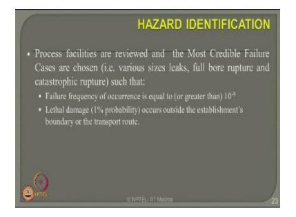
Let us now see what are different hazards identify in the group guide and session in different segments marked as 1 to 9 in the process flow diagram the process facilities are carefully reviewed and the most credible failure cases from the process industry as in case of this case as group gathering station is carefully chosen now when we ask the question what are those most credible failure scenarios which are chosen for the present study various sizes if week ages full bore rupture.
