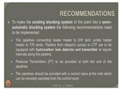
So the final recommendations given to the study are the following to make the existing blocking system of the plant in the semi automatic the following recommendations need to be implemented the pipelines connecting heater treated to E/R tank jumbo heater treater to E/R tank pipeline dispatched pumps to CTF are to equipped with hydrocarbon leak detector and transmitters at regular intervals how long length of the pipeline which is given in the present study.
