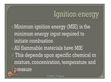
Having understood this let us see what we mean by ignition energy this is a minimum energy which is an input required to initiate a combustion in a given reaction all flammable materials have something called minimum ignition energy which is available in the chemical engineering handbook which will show you an extract in the next slide of course the minimum ignition energy depends upon specific chemical or the mixture it is concentration temperature and operational pressure.
