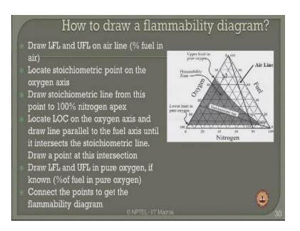
Now the question interesting comes how do I draw a flammability diagram to start with Flammability diagram is a triangular-shaped figure there is got three arms nitrogen, fuel and oxygen the concentration of them in every arm varies in a specific style 0 to 100, 0 to 100, 0 to 100 in an anti-clockwise manner for a given percentage fuel in air try to mark the lower flammability and upper flammability of fuel on the airline.
