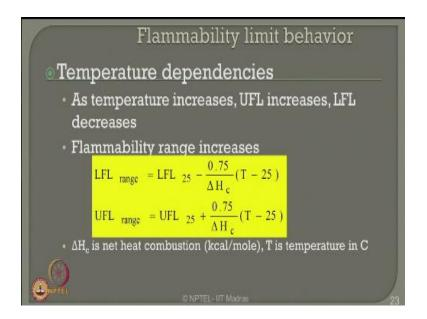
Can also work on the LFL and t UFL ranges directly from the flammability limit behavior let us quickly see what is the temperature dependency of the flammability limits as the temperature increases friends you saw in the last figure UFL and LFL decreases UFL increases therefore the range of the flammability keeps on broadening the flammability range therefore increases you can also work out this range from the equation shown in the slide now.
