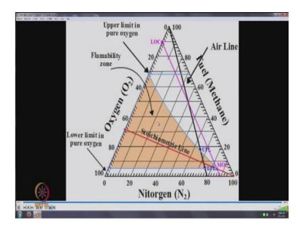
I play this once again nitrogen arm the fuel arm the oxygen arm is an order anti-clockwise airline seventy-nine percent nitrogen stoichiometric point taken from the reaction equation LFL UFL marked on the airline LOC marked on the oxygen arm draw a parallel to the fuel arm intersection of turkey will give MOC, LFL and UFL on the oxygen arm will me the boundaries and join this to get the flammability region hatch them to get the flammability region is what we call as a flammability diagram.
