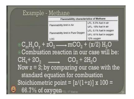
We will take an example of hydrocarbon problem which is methane which is ch4 now for methane the flammability characteristics are available in the literature as follows the flammability limits in air that is lower and upper is about 5.3 and 15 fuel in air whereas the flammability limits in pure oxygen is about 5.1 percent fuel in oxygen and 61 percent fuel in oxygen the limiting oxygen concentration below which methane will not catch fire is about 12% of oxygen.
