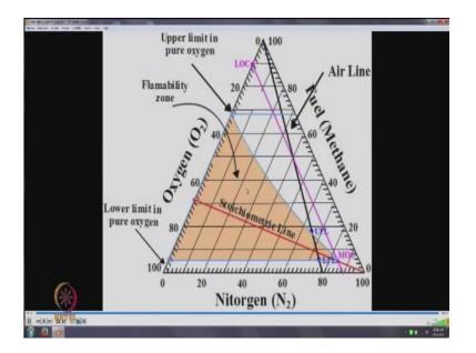
Now let us see a video quickly how to draw a flammability diagram the arm of the see is horizontal is a nitrogen arm 0 to 100 followed by which you draw the fuel arm which is methane 0 to 100 then the oxygen the prepare a grid select the apex of oxygen draw the airline then mark the stoichiometric point draw the stoichiometric line mark the UFL and LFL on the airline.
