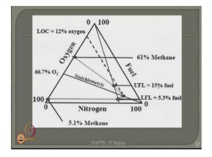
One similar stoichiometric point I draw the flammability diagram like nitrogen arm fuel arm and oxygen arm mark the airline which is apex or zero of oxygen is there are 79 percent of nitrogen which is called as an airline on the airline mark LFL and UFL of the fuel in air.
