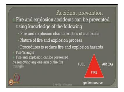
Now the essential question comes after understanding basic characteristics of fire and explosion how can we prevent the fire or an explosion accident now if we look at this triangle which is shown on the screen now this is famously known as fire triangle is fire triangle has got three arms one is the oxygen arm the other is a fuel alarm the third one is the ignition source hypnotically friends if any one of this arm is not present it will not result in fire.
