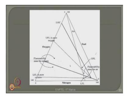
Which is again shown in the same manner so the flammability region in the specific example is what is shown between the dotted lines here this is the line which is limiting oxygen concentration which is marked on the oxygen arm and line drawn parallel to the fuel arm flammability diagram has got an order nitrogen fuel and oxygen market anti-clockwise 0 100, 0 100 and 0 100.
