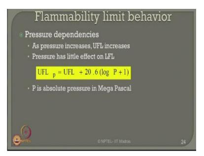
Flammability also depends on pressure as pressure increases the upper flammability increases however the pressure has very little effect on lower flammability this can also be directly obtained from the equation shown in the slide now where P is absolute pressure in mega Pascal.
