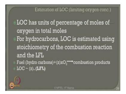
As I said it is very important to also know what is the limiting oxygen concentration because below distant oxygen concentration the fuel will not catch fire LOC has units of percentage of moles of oxygen in a total mole for hydrocarbons LOC is estimated using stoichiometric balance of a combustion reaction and the LFL hydrocarbons plus oxygen concentration gives me the combustion products loc is nothing but the oxygen concentration of the top LFL. (Refer Slide Time: 27:40)
