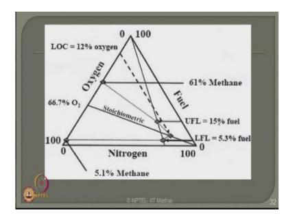
So mach twelve percent on the oxygen arm draw a line draw a line parallel to the fuel arm wherever this line and the stoichiometric line intersects mark the point and extend the LFL and UFL points now you get the values intersections as a b c d and e which is nothing but if 5.1 % methane and 61% methane on the oxygen arm which are available here.
