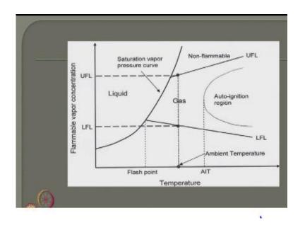
Let us quickly see this particular figure which is shown in the slide the figure plots the variation of temperature verses flammable concentration and there are two limits mark in the y axis which is lower flammability and upper flammability limits within which or between which the liquid or the fuel remains flammable beyond which and below which the fuel is not flammable that is why we are marked as non flammable beyond this region.
