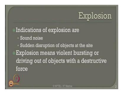
Let us quickly understand what do we mean by explosion explosions are generally indications measures of sound noise and sudden disruption of objects at the site expression means violent bursting or driving out of objects that the destructive force so therefore an important concept in explosion is that what is the quantum of energy being released when a material or a chemical mixture is exploded.
