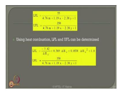
So LFL and UFL can also be obtained from the heat combustion equations as shown here where m x and y will be as same as what we explained in the last slide.
