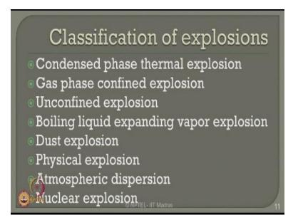
Explosions can also be classified further based on condensed phase thermal explosion gas phase confined explosion unconfined explosion boiling liquid expanding vapor explosion what we call BLEVE dust explosion, physical explosion and atmospheric dispersion which is also a form of or a kind of explosion. Nuclear explosion is of course a rare phenomena but however the disaster cost because of these explosions or very catastrophic and the societal damage arising from such are very severe.
