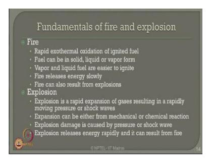
Therefore to model them let us try to understand few technologies in basics of fire and explosions fire is a rapid XO thermal oxidation of any ignited fuel this fuel fortunately can be either a solid or a liquid or even in a vaporous form the vapor and liquid fuel or of course easier to ignite compared to the solid ones when it catches fire it releases energy slowly there is no sudden release of energy in case of fire.
