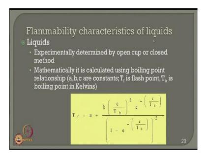
The flashpoint of the liquid even though experimentally this can be also computed directly by an open cup or a closed cup method.
