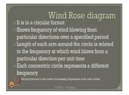
The wind rose diagram is in a circular format in general it shows frequency the wind blowing from a particular direction over a specific period. Length of each arm in a given circle is related to the frequency at which the wind blows from a particular direction per unit time. Each concentric circle as a set beginning it represents a different frequency it starts from 0 at the center which is a calm state to an increasing frequency as moves towards the outer circles.
