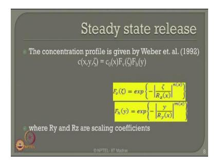
When we talk about the steady state release then the concentration profile is given by the following equation. Where the concentration in terms of x,y and z coordinates are given by the equation as you see in the slide here, whereas  $F_v$  and  $F_h$  are subsequently exponential expressions I see from here where in this expression  $R_y$  and  $R_z$  are the scaling coefficients which are relatively applied along the y and z axis respectively in this equation.
