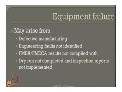
The third subset which comes from equipment failure may arise from defective manufacturing engineering faults not identify why equipment manufacturing stage itself failure mode effect analysis or failure mode affect criticality analysis are not complied with the proper results and recommendations made by these analysis, dry run not completed and inspection reports not implemented in the equipment manufacturing stage itself.
