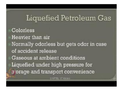
As a first case we talked about liquid petroleum gas which is LPG when I important characteristics of LPG which we all know but still as a summary let us present it here generally it is colorless it is heavier than air normally order less that gets water in the case of accident release it is generally gaseous at ambient conditions is liquefied under high pressure for storage and transport conveniences LPG.
