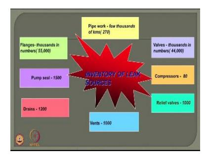
But focus on the connections which are very important because they are seemed to be a potential challengers for leak in any given process industry.
