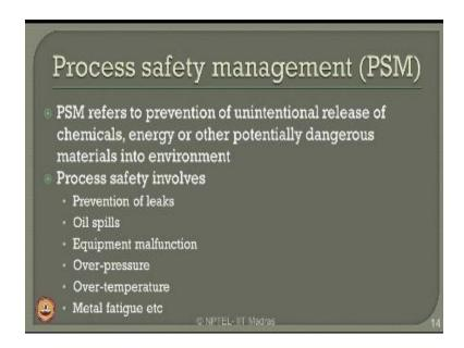
Therefore the integrated feature of process safety is managing the whole issue what we call as process safety management. Process safety management refers to prevention of unintentional release of chemicals, energy or other potentially dangerous materials into environment. Process safety of course involves prevention of leaks, prevention of oil spills, prevention of equipment malfunction, avoiding overpressure, avoiding over temperature, avoiding metal fatigue extra.
