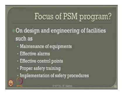
Therefore, what should be the focus of my process safety management program? On design and engineering of facilities I should focus on of course maintenance of equipments in a periodic cycle, I should also design effective alarms and signal generator systems in a given process industry. I must establish effective control points where I can check the leak or at least the extension or spread of the leak if the leak has occurred.
