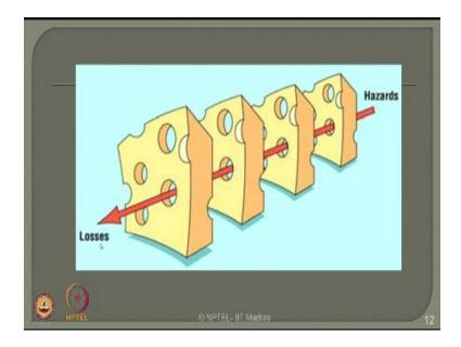
Now this picture shows how hazards which are scenarios will result in potential losses which becomes an economic threat to the company. So when the holes which are nothing but imperfections which are violations of standards at different stages in process industry, when they all get aligned a simple hazardous situation can become a serious potential loss or economic loss to the company itself.
