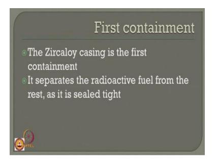
Let us talk about different containments in nuclear reactor the first containment is the Zircaloy casing it separates radioactive fuel from the rest because this is completely sealed tight.
