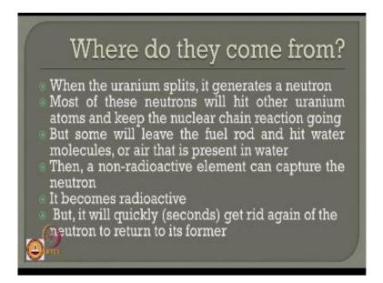
Another question comes where these elements come from? When the uranium splits it generates a neutron most if these neutrons will hit other uranium mattes and keep the nuclear chain reaction going on, but some will leave the fuel rod and hot water molecules or air that is present in water then a non radioactive element can capture the neutron it becomes radioactive, so there is a catch here even though when the uranium splits and generates neutron.
