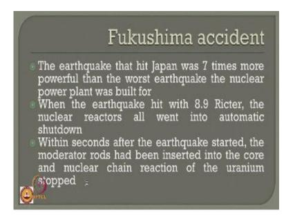
So within seconds after earthquake occurred moderator rods has been inserted into the core as a nuclear chain reaction of the uranium was stopped, so one can say this is the first line defense of safety by design.
