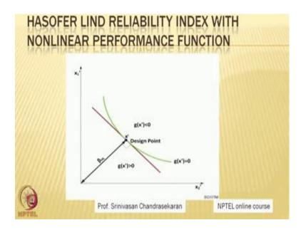
The screen shows the graphical representation of 2 variables; x 1 bar and x 2 bar, which is going to govern the limit state function and the performance function as suggested by Hasofer Lind reliability index of course, you can see here the performance function is non-linear which is shown in the green colour. So, g x prime is equal to 0 that is my limit state function or performance function.
