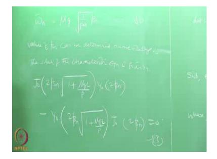
The frequency omega bar n will be given by u g 1 by P M of beta n; equation number 12. Now the value of beta n can be determined numerically, because the solution of the characteristic equation is given right, that is the reason why we can get beta n numerically J 0 2 beta n 1 plus u g l by P Y 0 2 beta n minus Y 0 2 beta n root of 1 plus mu g n by p J 0 2 beta n said to 0; equation 13. Substituting the value of the above equation in the original equation of motion what we had.
