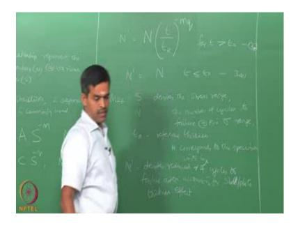
At this stress range t R is call the reference thickness and N corresponds to a specimen with t R. N dash of course denotes reduce number of cycles to failure after accounting for shell or plate thickness. In this case t plate thickness effect t. A denotes fatigue strength coefficient, m and r are fatigue strength exponents.
