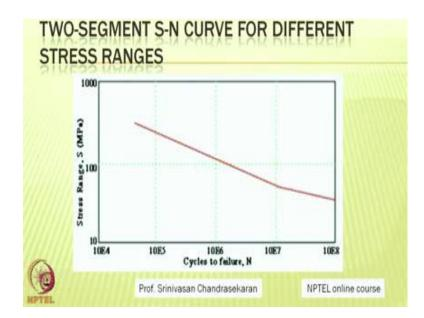
One can see here S is plotted as a stress range in mega Pascal in the vertical scale on axis and the cycles to failure N is plotted in the horizontal axis varying from 10 to the power 4 to 10 power 8 cycles. The red line shows actually the 2 segment S-N curve - one segment is this, other is this, whose slope is different therefore that line is discontinuous at N equals N Q.
