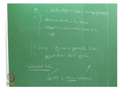
That's the question now the answer is yes we can do the study is named by a specific character that is called failure more and effect analysis what we abbreviate as FMEA, FMEA will be able to analyze the mechanical faults in the design, but it requires at least a scaled model a scaled working model of the system now I want to actually analyze in the in the design stage itself a process line, how do I do it then in that case you can do
