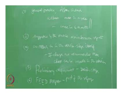
Hazop studies are generally carried out to identify the potential hazards and operability problems passed over the deviations those arise from the design intent. In particular, if there are major deviations present or they are made in any recent modifications of the plant then the hazop should be conducted. One, if any major modifications are done to the flow line of the plant then one should do hazop report, hazop study.
