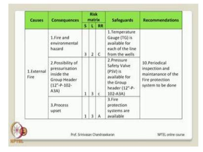
Because you know temperature is one of the important sources which can cause fire. So, high temperature will result in external fire. You have a fire environmental hazard,
