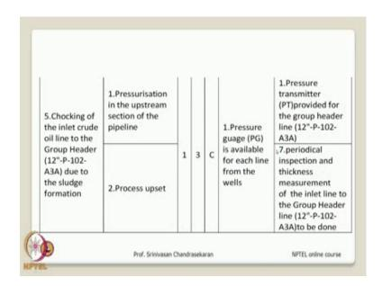
Let us move ahead, 5th cause could be choking of the inlet crude oil line. Pay attention to the screen. Now it will result in pressurization, it can cause process upset, it has severity and likelihood on a scale of 1 and 3 like this, the risk ranking refers to C, pressure gauge is available in the safeguard already which can tell me whether the pressure is extent is dangerous beyond limit or not.
