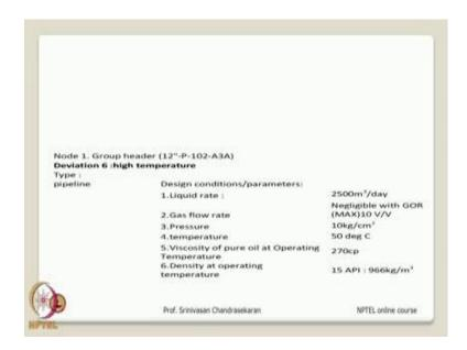
The second the next can be a deviation 6 which is high temperature - high temperature will result in external fire.
