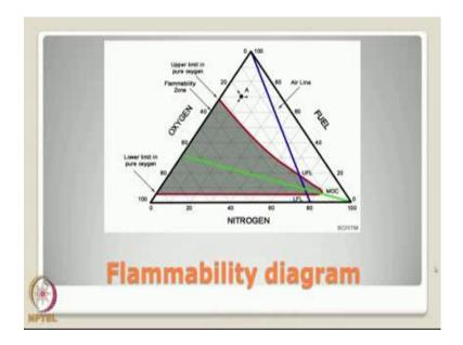
You will get a typical diagram of the flammability diagram shown in the screen which is as same as what I explained in the black board here.
