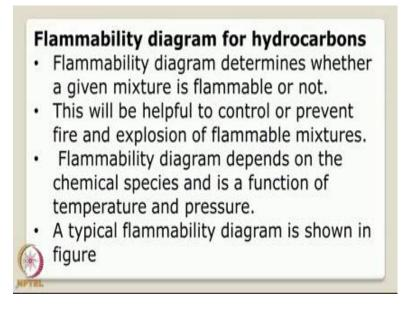
So, flammability diagram is useful in understanding whether the fuel mixture is flammable or not.
