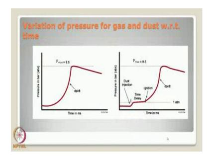
The left side figure shows the variation of pressure for gas respect to time, whereas the right side figure shows the variation for dust. So, the pressure gradient is different in case of a gaseous release on an explosion caused by gas compared to that of dust.
