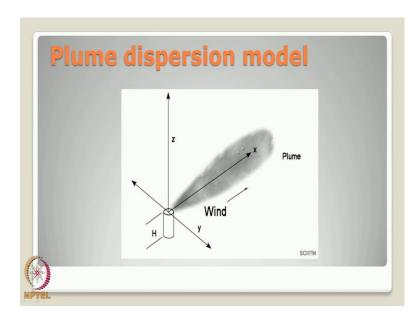
Which is a classical plume dispersion model used in the literature as explained. This is the point of release of the gas which is at a constant height H from the ground and the wind is blowing predominantly in the direction along the x-axis.
