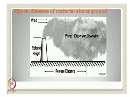
The figure shows release of material above ground. So, one can see here, if this is chimney or a stack, this is realizing the gas into the atmosphere and if this is a predominant wind direction as you can see from the wind rose diagram, one can see the released vapor or the gas goes high and it takes a specific distance to touch the ground. It means this is what we called as released distance.
