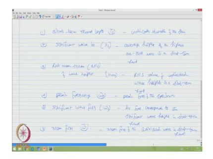
Let us say short term record length, it is Ts, which indicates the duration of strum; significant wave height Hs, which is average height of highest one-third wave, in a short term record root means square that is rms of wave height, which we called H rms, this is root mean square value of individual wave heights in a short term record.
