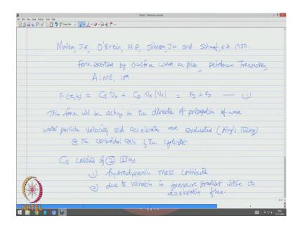
Force exerted by surface waves on pipes petroleum transactions AIME 189. So, according to them F of z t is C I, V dot x plus C D, V x V x which is inertia term plus (Refer Time: 26:52) term. This force will be acting in the direction of propagation of wave that is in the forward direction.
