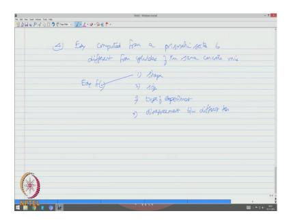
The forth factor dynamic modulus of elasticity computed from a prismatic section is different from cylinders of the same concrete mix. So, E dy is function of 1 shape, 2 size, 3 type of experiment and forth a strong disagreement between different test. So, there is a wide variation. Let us see one by one by different test how E d can be calculated.
