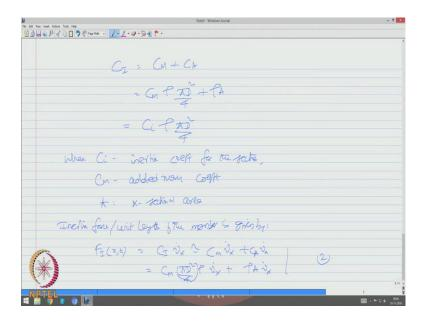
As C i rho pi D square by 4 where, C i is the inertia coefficient for the section, C m is the added mass coefficient, A is the cross sectional area therefore, inertia force per unit length of the member is given by F I, again a specific location z t is C I V x dot is approximately C m V x dot, plus CA V x dot, which can be C m pi D square by 4 rho V x dot, plus rho A V x dot - let us call this as equation number 2.
