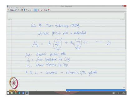
So, according to two-frequency method, dynamic poisons ratio is estimated, which is given by A1, f 2 by f 1 square plus B1, f 2 by f 1 plus C 1 where mu d is called dynamic poisons ratio; f 1 is the first longitudinal frequency in hertz, f 2 is the second resonance frequency in hertz A 1, B 1 and C 1 are actually constants, which depends upon the dimensions of the cylinder.
