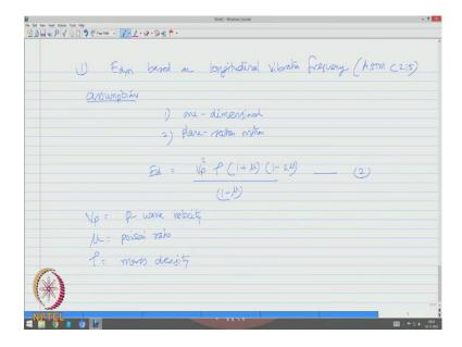
Let us say E dyn based on longitudinal vibration frequency. Please understand dynamic modulus depends on very strongly the type of (Refer Time: 15:06) you perform. This is as per ASTM C215, it has got some basic assumptions, the test is performed on one-
