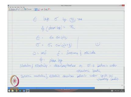
So, strain is E0 sin omega t, where as stress is sin 0 sin omega t plus pi and we know omega is 2 pi f, where f is a frequency of oscillation and phi is called as phase lag. Generally modulus of elasticity is described or let say defined as stress strain behavior under monotonic loading, where as dynamic modulus of elasticity describes behavior under cyclic or vibratory loading.
