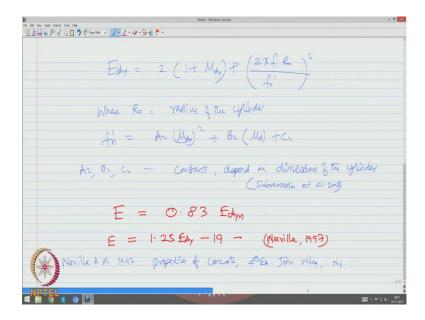
Once I know the dynamic poisons ratio, I can find dynamic modulus of elasticity as twice 1 plus mu dynamic rho, 2 pi f 1 R 0 by f n dash square where, R 0 is the radius of
