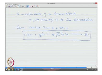
For surface elevation eta be a Gaussian distribution, V that is water particle velocity will also follow Gaussian distribution. Hence linearized Morison equation is given by F z of t, C i V x dot, plus C D root 8 by pi sigma V x, V x equation 4. So, that is the linearized term what we have, which is again an approximation of one important drag non-linearity coming down from the equation.
