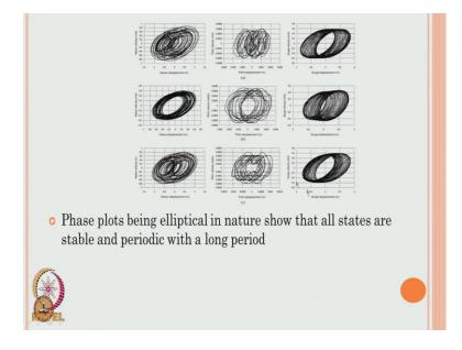
Now, to look at the stability of the system, one is interested to plot the phase plots, the phase plots in heave degree, pitch velocity or pitch degree and surge degree in terms of velocity and displacement for all the 3 TLP's, TLP 1, TLP 2 and TLP 3 show more or less they are elliptical in nature with a shift in the major axis. Elliptical in nature in heave degree of freedom which is a stiff degree clearly shows that they are stable and periodic with a long period.
