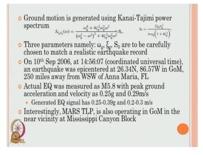
The ground motion generated is in Kanai Tajimi power spectrum is given by this equation, where the power spectral density function of the ground acceleration is given by this equation, where S 0 is what we call as an intensity parameter. So, now, this particular equation is to be actually chosen with 3 requirements.
