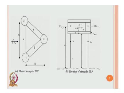
We will now apply this to a geometric optimization of a triangular TLP which is got 3 column members named as 1 2 and 3 and 3 (Refer Time: 42:45) members named as 4, 5 and 6 and the elevation of this is shown on the right hand side screen for you. So, equivalency of a triangular configuration is arrived by comparing its characteristics with an established constructed square TLP's.
