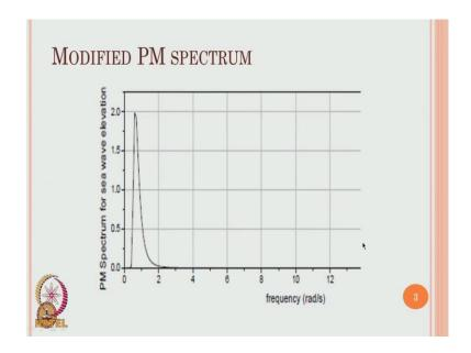
Let us now see how the modified spectrum looks like. The modified Pierson Moskowitz spectrum which is function of model frequency, which is chosen to be 5 times of that of such frequency, is shown in the sketch now on the screen.
