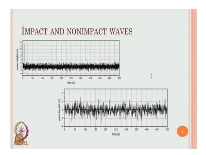
The generated or simulated impact waves and non-impact waves in terms of sea surface elevation, time history is shown on the screen, one can distinctly see at an impact wave as a special kind of wave height which is distinctly high compared to its predeceasing and successive waves in the entire history simulated whereas, in non-impact wave no such near vertical front configuration is required.
