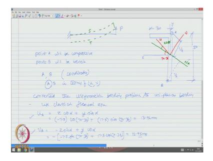
This is the given section, we have the z axis located here and y axis located here, uu axis located 70 degree, this angle is 70.36. We also located the neutral axis which is 22.88 degrees.
