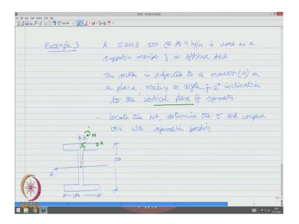
To understand this we will take an example, let us say example 3, A ISMB 500 at 86.9 kg per meter is used as a supporting member of an offshore deck this section is subjected to a moment M on a plane which is not matching with the axis symmetry, but making an angle of 2 degrees inclination to the vertical plane of symmetry. So, locate the neutral
